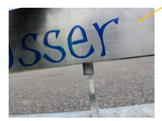
Place a straight edge on the element and take the measure at the deepest point.
