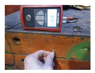
Place the material thickness device on a straight surface and take the measure. This test method is not suitable for frames. Please just use this method at thicker elements. The workers which uses this test device should be instructed in using this.
