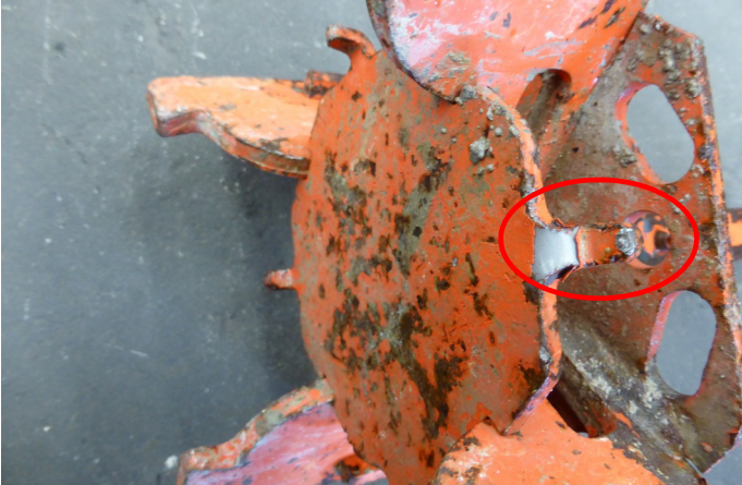
21.23 Pieces torn out
